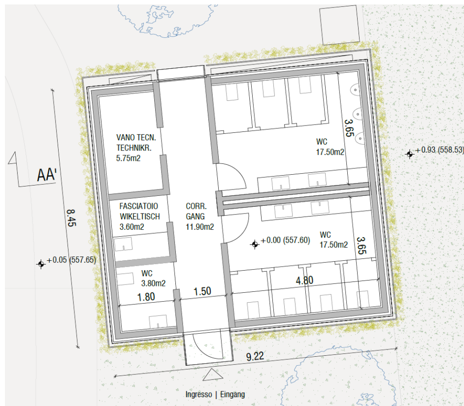
ERDGESCHOSS | PIANO TERRA
